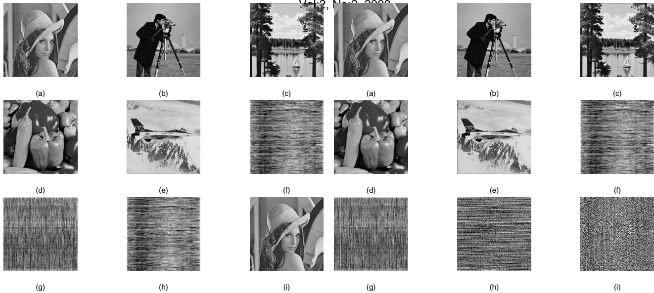
Fig. 8. Results of encryption by magnitude and phase manipulation using carrier images. (a) Original image, (b), (c), (d), (e) different carrier images, (f) encrypted image by row wise operation, (g) encrypted image by row and column wise operation, (h) decrypted image by column wise operation and (i) decrypted image by column and row wise operation.
