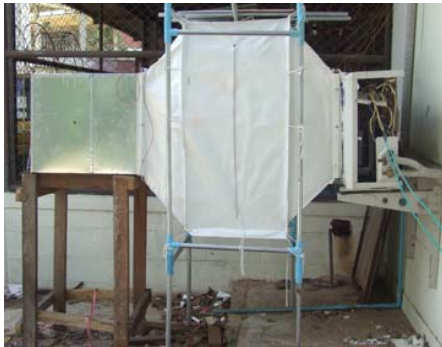
Fig. 3 Clothes drying chamber installed to the condensing unit
