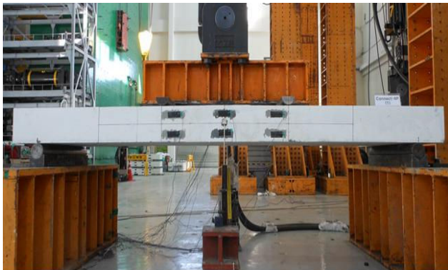
Fig. 5 Bending test setup
