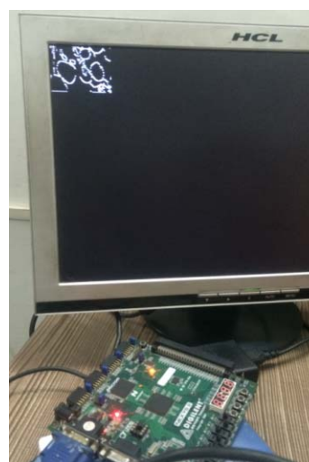
Fig. 9 VGA screen with Xilinx Vertex 4 development board
