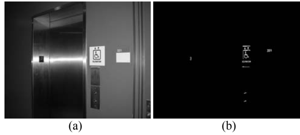
Fig. 16 Results of images with single character and strong reflections (a) Original images (b) Extracted text
