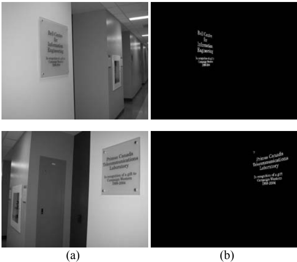
Fig. 14 Results of images with strong reflections and different perspective distortion (a) Original images (b) Extracted text
