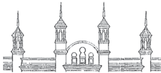
Fig. 25 Parapet wall with miniature chattris acts as a pinnacle (VOT 69651, KALAM)
