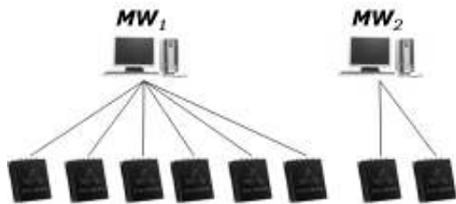
Fig. 2 RFID middlewares with the connected RFID readers
