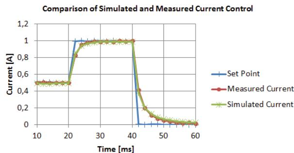
Fig. 4 Comparison of Simulated and Measured Current Control
