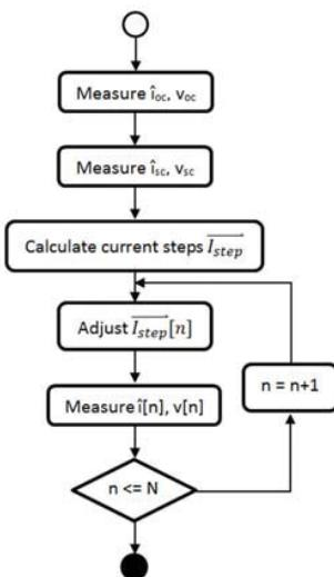
Fig. 5 State diagram of measurement function
