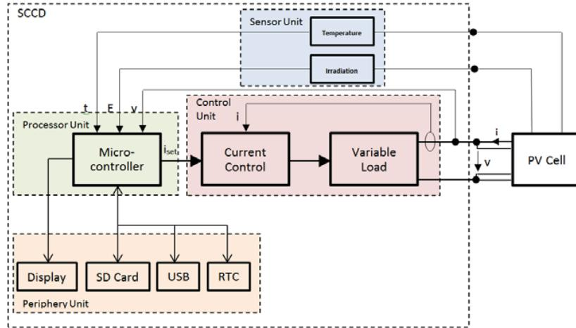
Fig. 2 Block Diagram of the Hardware Design
