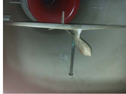
Fig. 6 Wind -Tunnel Model in Yaw Attitude
