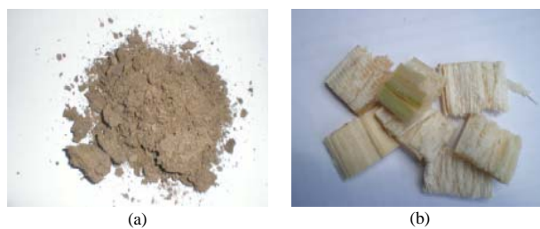
Fig. 1 The agricultural residue biofilter media (a) manure fertilizer (b) bagasse
