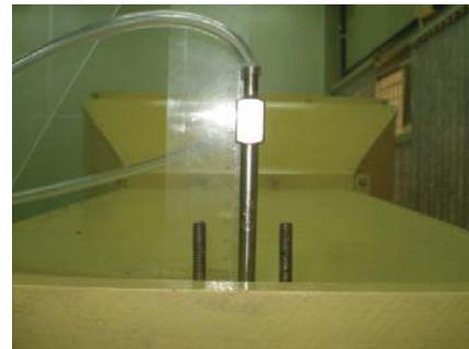
Fig. 4 Height adjustment of the Pitot tube
