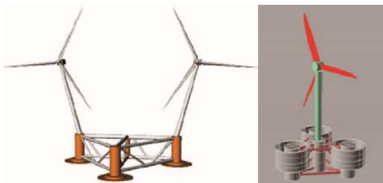
(a) twin turbine structure [49] (b) single turbine tripod [50]
