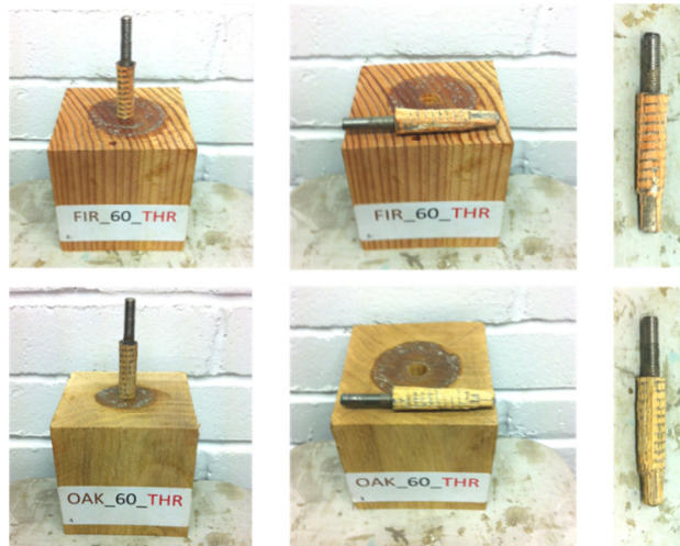
Fig. 13 Failure mode in Oak (bottom) and Douglas Fir (above) samples with rough and threaded borehole after being tested by a pull-out test
