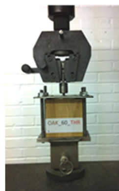
Fig. 8 Pull-out testing machine
