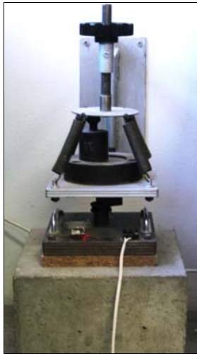
Fig. 3 Measurement of dynamic stiffness
