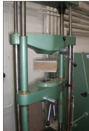
Fig. 2 Measurement of tensile strength
