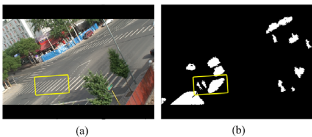
Fig. 8 Pedestrian-vehicle traffic conflict detected by improved algorithm: (a) subtracted background; and (b) extracted moving objects
