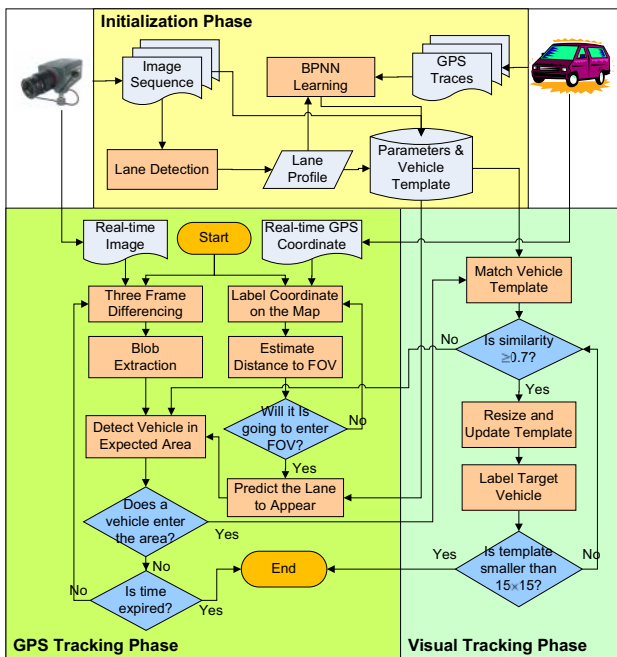
Fig. 3 The operation process of GPS-VT for vehicles
