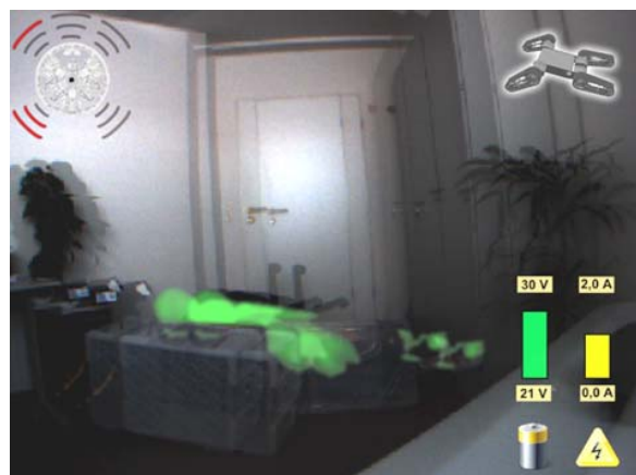
Fig. 11. Example of the stereo sensor fusion. The highlighted part in the center corresponds to a trapped person. Additionally, the stereo stream is enhanced with further mono GUI overlays.
