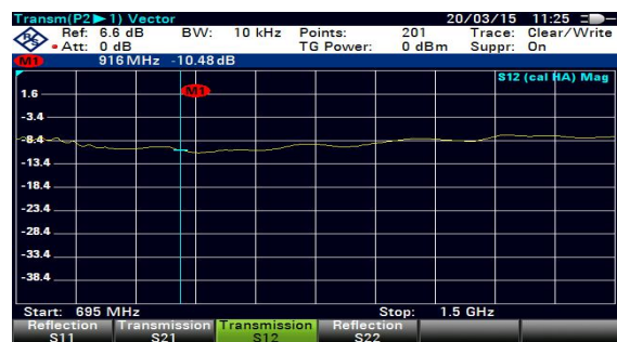
Isolation loss S_{23} = -10.48\text{dB}
