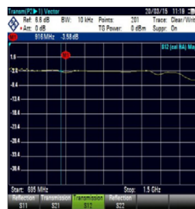
Insertion loss S_{12} = -3.58\text{dB}
