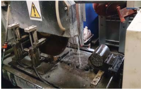
Fig. 7 Asphalt Specimen Undergoing Slab and Core Drill [7]
