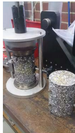
Fig. 10 Final Asphalt Specimen [7]
