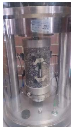
Fig. 11 Final Asphalt Specimen in AMPT [7]
