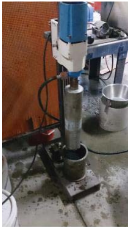
Fig. 6 Asphalt Specimen Undergoing Core Drill [7]
