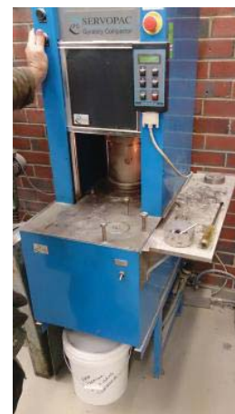
Fig. 5 Gyratory Compaction of Asphalt Specimen [7]
