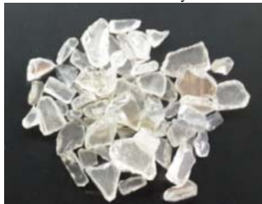
Fig. 1 (b) The crushed CRT glass as coarse aggregates used in this study
