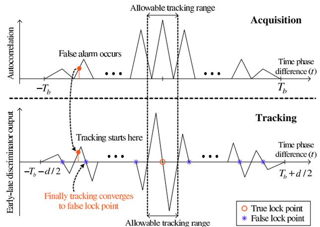
Fig. 1. Ambiguity problem in BOC signal synchronization.
