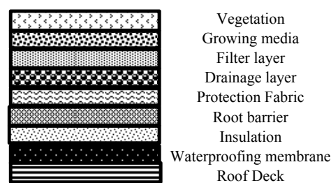
Fig. 1 Structure of green roof system
