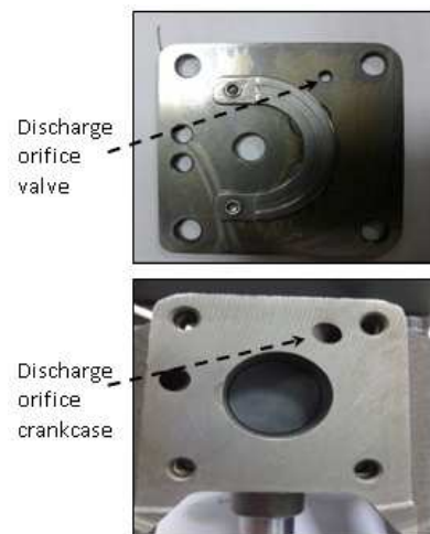
Fig. 3 Discharge orifice of valve plate and crankcase
