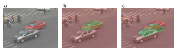
Fig. 7 Impact of incorporating the silhouette-based measure on vehicle matching: (a) Test image, (b) Matching result with the incorporation of the silhouette-based measure, (c) Matching result without the incorporation of the silhouette-based measure
