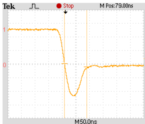
Fig. 9 Experimental reverse recovery waveform at di/dt=100A/\mu s , I_F=1A , V_R=30V , (0.4A/div, 50ns/div)
