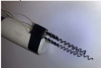
Fig. 10 testing model for multi-flagella propulsion concept
