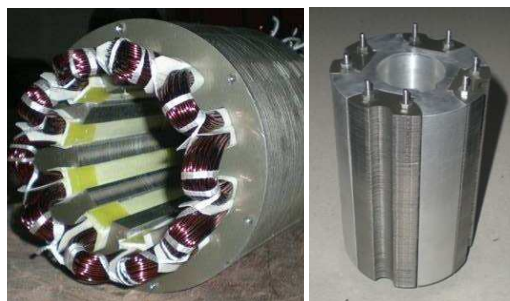
(a) Front views of the stator and rotor before they are joined to other parts and placed into frame
