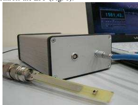
Fig. 1 The dosimetry system: phototransistor on a printed circuit board, the Flip-flop electrometer, a computer and the DoseX ® software
