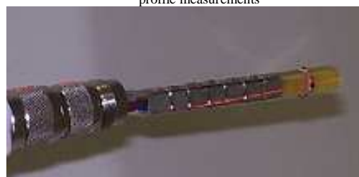
Fig. 5 Detector configuration with four phototransistors, mounted with right angles between each phototransistor
