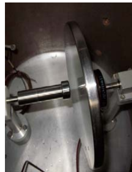
Fig. 2 Stainless Steel electrodes: Rogowski/plane electrode configurations
