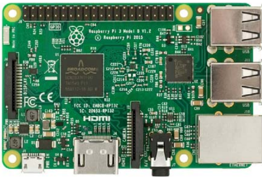
Fig. 1 Picture of a Raspberry Pi 3 Model B
