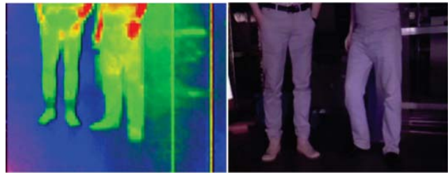
Fig. 12 Comparison of IR and normal camera images
