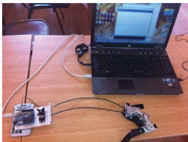
Fig. 13 Knee modular orthosis prototype with attached command&control unit
