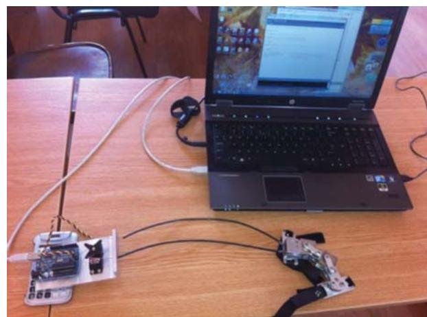
Fig. 13 Knee modular orthosis prototype with attached command&amp;control unit
