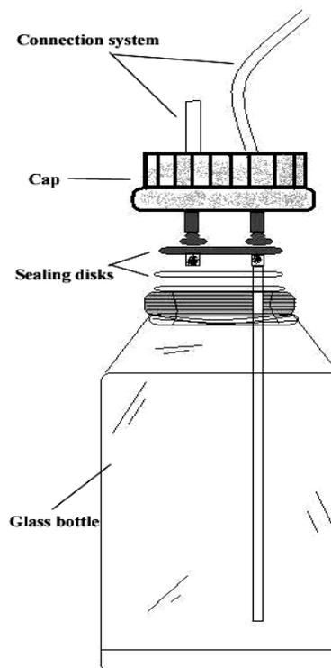
Fig. 2 Connections in an air-tight laboratory bottle
