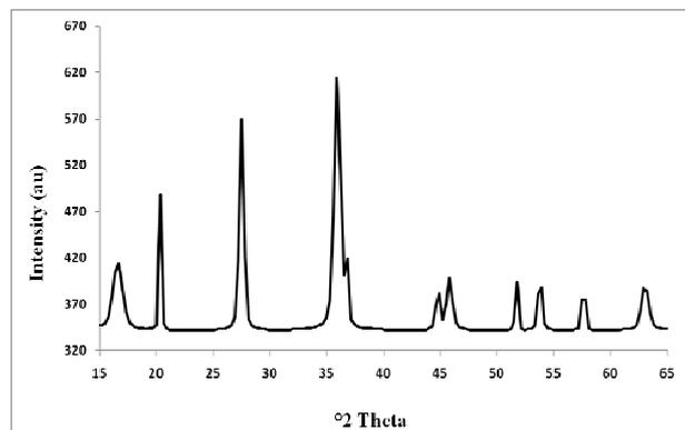
Fig. 5 XRD diffraction patterns of isolated magnetosomes
