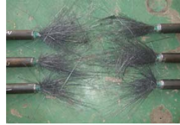
Fig. 9 Failure pattern of 3-multi CFRP tendon
