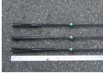
Fig. 7 3-multi CFRP tendon
