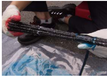
Fig. 8 7-multi CFRP tendon
