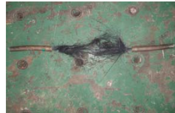
Fig. 11 Failure pattern of 7-multi CFRP tendon
