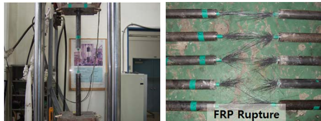
Fig. 5 View of tensile test and failure pattern
