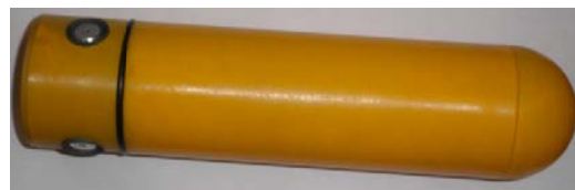
Fig. 8 Prototype micro communications sonobuoy
