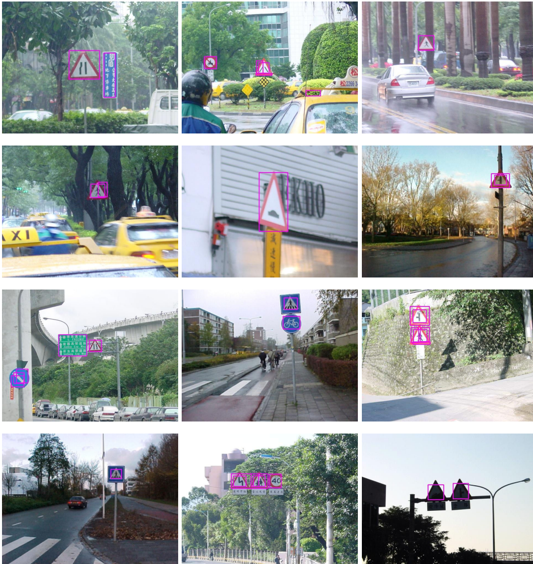
Fig. 6. Some examples of the experimental results using proposed sign localization method.
