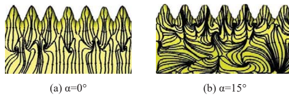
Fig. 9 Friction lines along 16L hydrofoil upper surface at \alpha=0^\circ and 15^\circ
