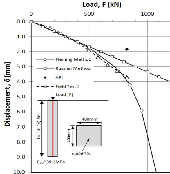
Fig. 5 Settlement comparison for the first tested pile
