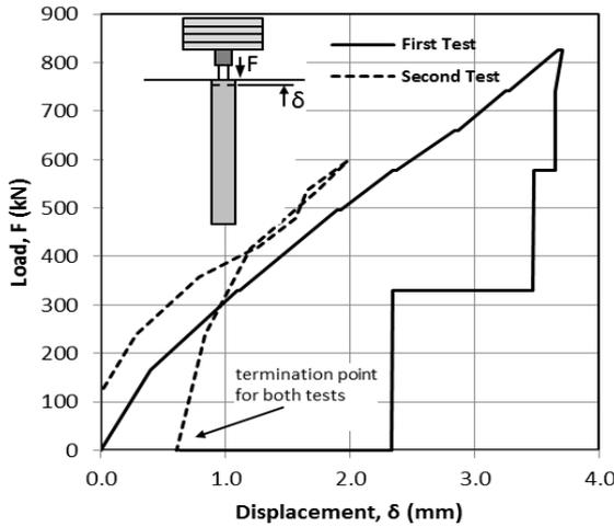
Fig. 4 Static pile test result
