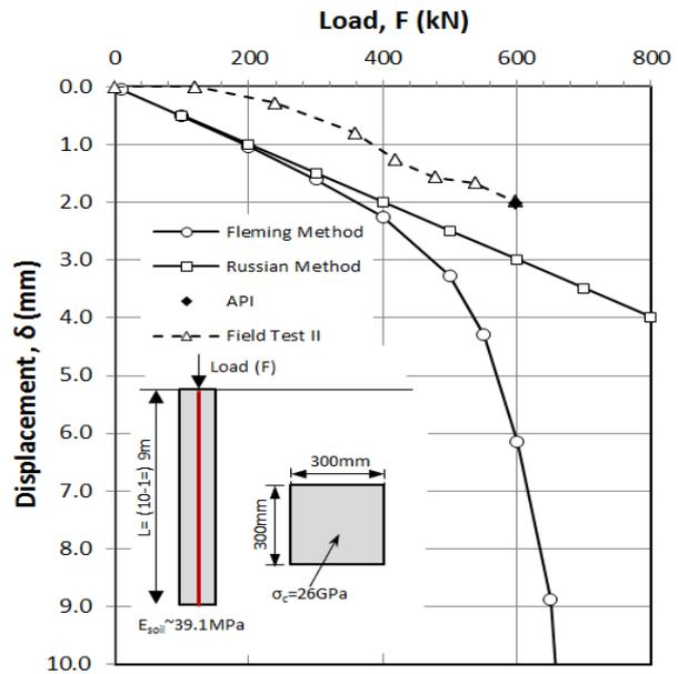
Fig. 6 Settlement comparison for the second tested pile
