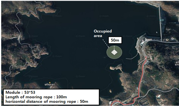
Fig. 2 Installation position of substantiation-plant
