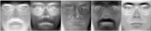
Fig. 1. The first five leading eigenvectors of the covariance matrix of the training data - first five Eigenfaces
