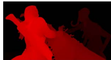
Fig. 9 One form of z-depth, which is stored in R channel of a projected image through a 3D stereoscopic camera
