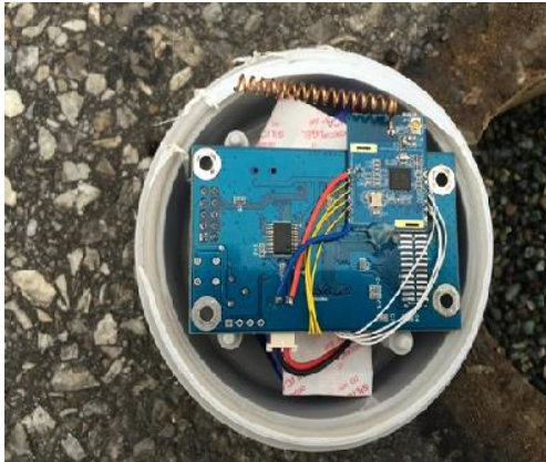
Fig. 5 The sensor node in enclosure
