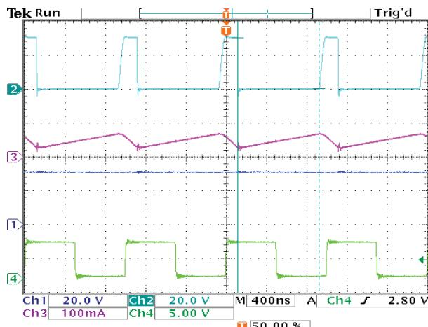
Fig. 10 Switching waveform at 5-mA load condition
