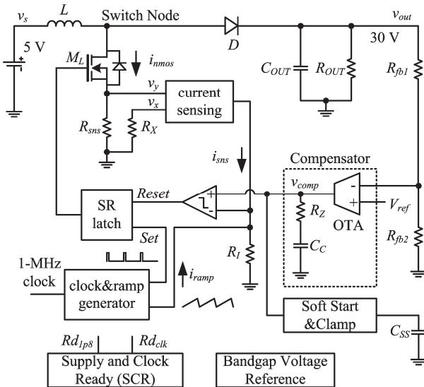
Fig. 1 Block diagram of the current-mode boost converter
