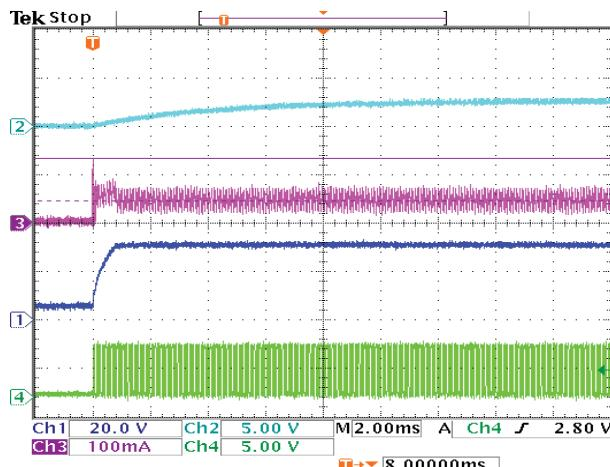
Fig. 9 Start-up waveforms,  $C_{SS} = 8.2 \text{ nF}$
