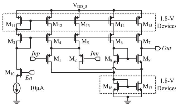
Fig. 3 Circuit schematic of the folded-cascode OTA
