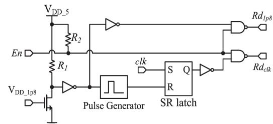
Fig. 4 Circuit schematic of the SCR block
