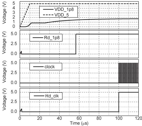
Fig. 5 Simulated signal waveforms of the SCR block
