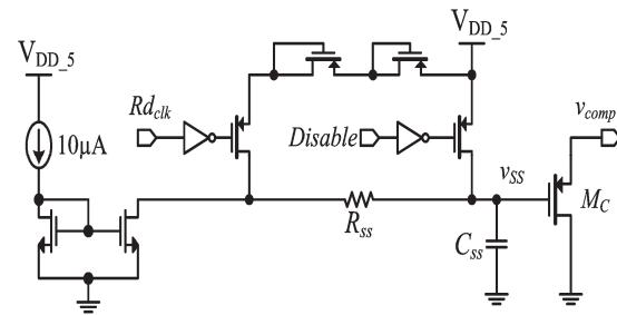
Fig. 6 Circuit schematic of the soft-start and clamp block
