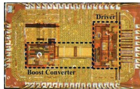
Fig. 8 Micro-photograph of the boost converter
