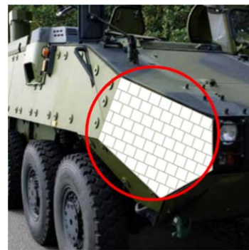
Fig. 2 Ceramic composite armor used for military vehicles [10]
