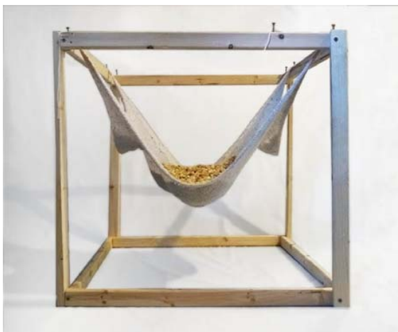
Fig. 5 Textile hung with rocks to weigh fabric into parabolic shape
