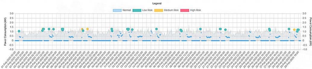
Fig. 4 Power Consumption with Predictive Range and Identified Anomalies in 10-hourly intervals
