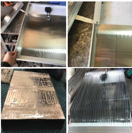
Fig. 3 Photographs of the fabrication process of the aluminum heat sink used in this study
