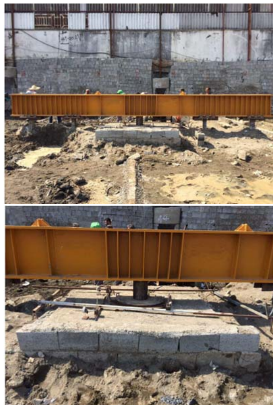
Fig. 3 Static loading test in south of Iran project
