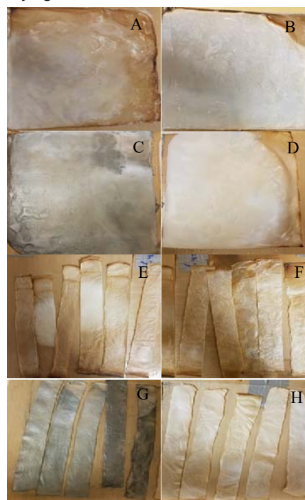
Fig. 2 (A)-(D) are dried C41, C42, C43, and C44 samples, (E)-(H) the tensile test specimens cut from C41, C42, C43, and C44 samples respectively
