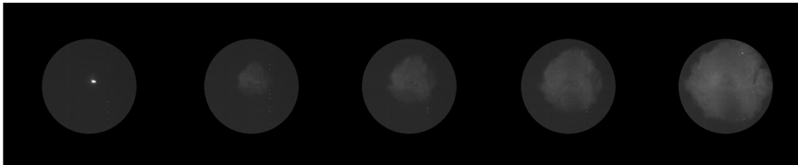
Fig 7 Representative sequence of the flame propagation process for the stoichiometric condition
